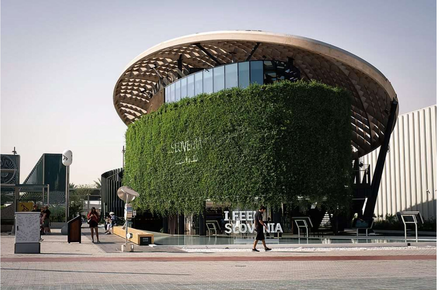
The pavilion of Slovenia has sustainably harvested spruce wood in its structure and roof, and it is wrapped in a green wall of 45,000 plants set in hundreds of meter-square panels of natural volcanic stone.
